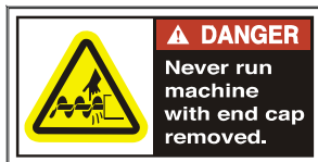
End Cap Label: located on discharge snout
