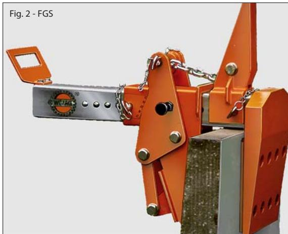
The Flat Grab FGS was developed for handling rough stones and concrete parts with parallel surfaces.
