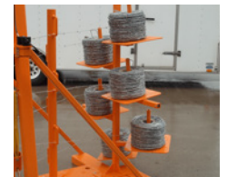
Concurrently dispense and tension up to six strands of barbed wire with optional SNGBARB attachment.
