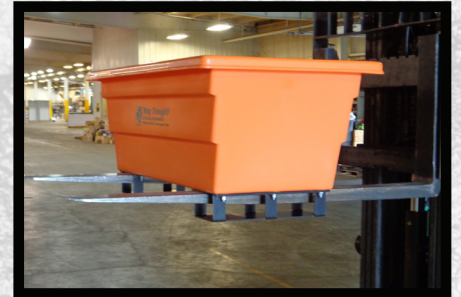
Steel legs can be lifted with forklift
