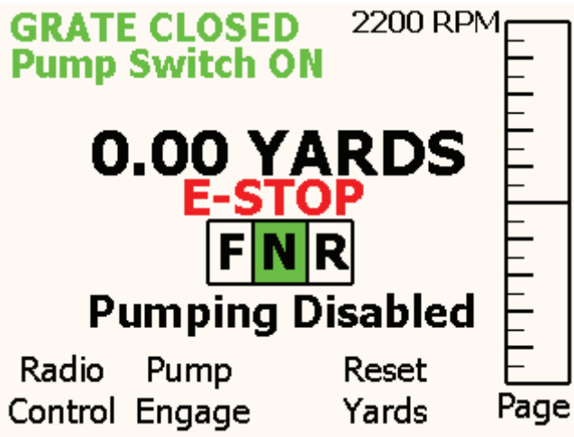
Figure 18 Pumping Disabled, Machine E-Stop Engaged
