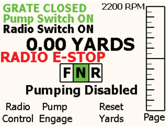
Figure 17 Pumping Disabled, Radio E-Stop Engaged
