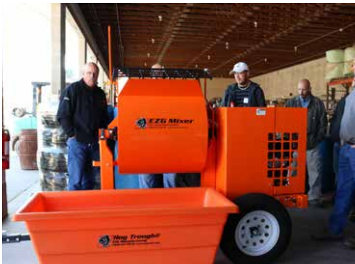
The EZG Mixers dump easily into the Hog Troughs or a wheel barrow without having to be raised on blocks.
