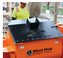
Optional solid grate cover, with two separate openings for adding mix and water, helps control dust on the job site.
