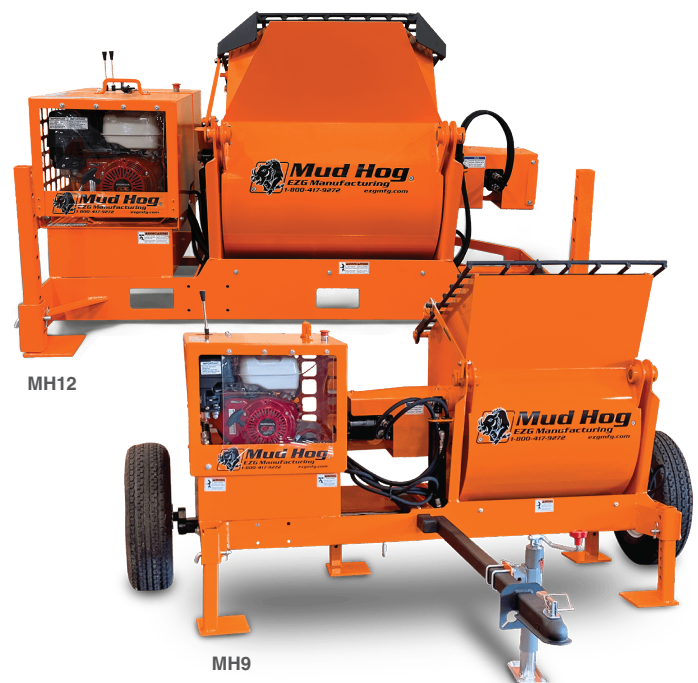
Forward / reversible mixing with patented vertical paddles and rubber blades prevents clogging, ensuring an optimal quality mix.
