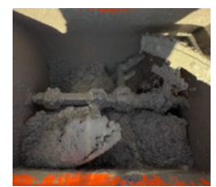
Hydraulic powered paddles with patented rubber blades for efficient clog-free mixing
